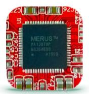
At the heart of Aquarius is its Merus<sup>TM</sup> amplifier - Infineon's most efficient audio amp. Merus boasts a stellar 92% efficiency, meaning that more of your battery's power is converted into sound and not into heat. More power savings means more hours of music giving Aquarius its 36+hour battery life at normal listening levels.
