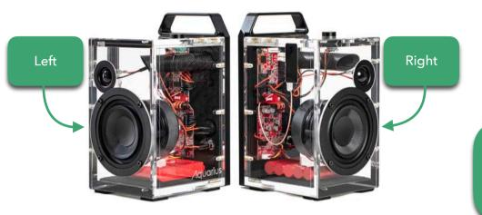
**Step 2:** Using the Master (left) speaker, hold down the Bond Button, then turn the speaker ON
