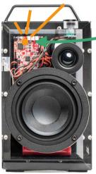
If the Bond Indicator stays dim Amber and there is no audio, Factory Reset by clicking the Bond Button 6 times. The Bond Indicator will flash Red if the reset is successful.
